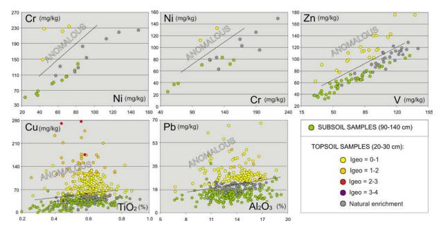
Fig. 20 – Detecting soil contamination with the aid of scatterplot diagrams. The green dots are representative of the pedogeochemical content. Coloured dots are inferred to represent metal contamination. The grey dots are interpreted as false positives (see text).
