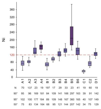
Fig. 12 – Natural distribution of Ni in the studied GFUs, with indication (in mg/kg) of the  $90^{th}$ ,  $95^{th}$  and  $50^{th}$  percentile values.
