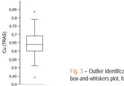
Fig. 3 – Outlier identification (white circles) for Cu in GFU B1, based on box-and-whiskers plot, following Box-Cox transformation (Fig. 2B).
