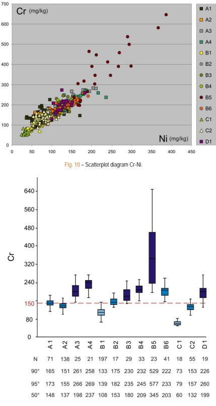
Fig. 11 – Natural distribution of Cr in the studied GFUs, with indication (in mg/kg) of the 90<sup>th</sup>, 95<sup>th</sup> and 50<sup>th</sup> percentile values.
