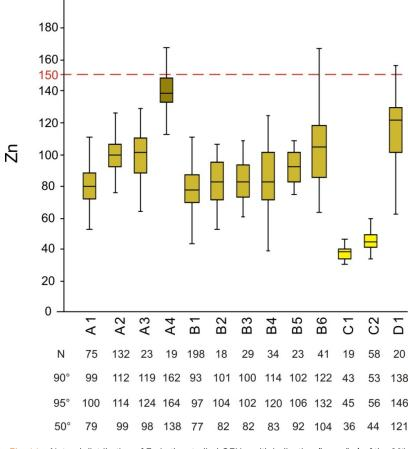
Fig. 14 – Natural distribution of Zn in the studied GFUs, with indication (in mg/kg) of the 90<sup>th</sup> , 95<sup>th</sup> and 50<sup>th</sup> percentile values.
