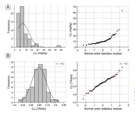
Fig. 2 – Example of frequency histogram and related cumulative distribution for Cu in GFU C2, before (A) and after (B) the Box-Cox transformation. The Box-Cox normality plot shows that the maximum value of the correlation coefficient is at  $\lambda$ = -0.2.
